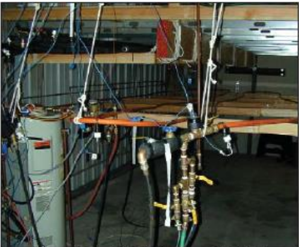
Figure 4. Test Rig for Uninsulated PEX-Al-PEX
