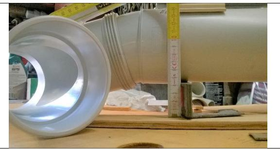
This image shows the approximate increase in pipework height is 43mm resulting from an increase in inclination of the junction by 15 degrees.
