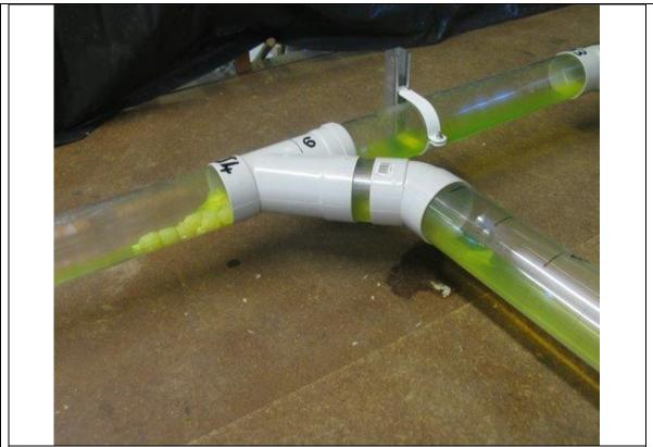
The image above shows the waste blockage/stranding at the 45 degree junction and up into the branch line in the standard test configuration
